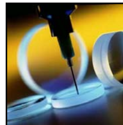
Ocular lens bonding
