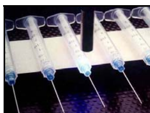
Automated syringe assembly
